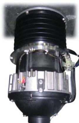
Anti-vibration mechanism (top) and Container (bottom)
